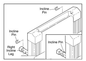
To change the incline, remove the incline pin from the right incline leg as shown below.
